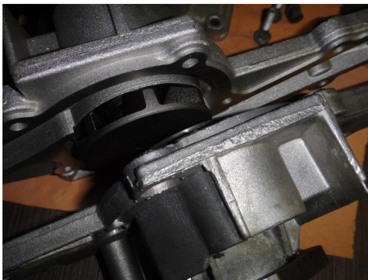
(Above the Magnetti pump, below the original Alfa pump)
