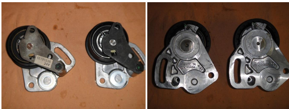
(In the photos: the Alfa tensioner on the right, and on the left the Litens from the Gates or SKF kits)
